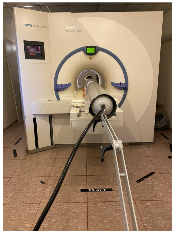
Figure 4.2.5: Waveguide and diathermy machine placement.
