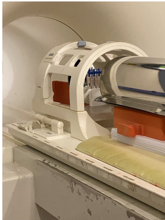
Figure 4.2.2: Placement of the solutions inside the head coil.
